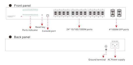
Attention 1: This product must be well grounded against lightning, please use better than 20# cable to connect the grounding terminal and ground.
